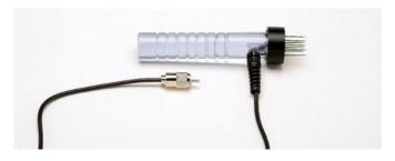
**37-E/C -** Used for yarn, 38 mm pins with 25 mm penetration.
